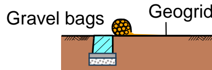
2) Placing gravel bags wrapped-around with geogrid
