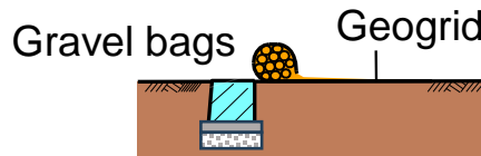
2) Placing gravel bags wrapped-around with geogrid
