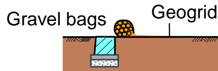
2) Placing gravel bags wrapped-around with geogrid
