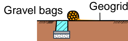
2) Placing gravel bags wrapped-around with geogrid
