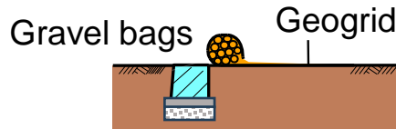
2) Placing gravel bags wrapped-around with geogrid
